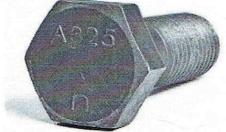
Grade 5 bolts are most typically made, and are most readily available in a <u>finished hex bolt</u> configuration. A325 bolts are required to have a <u>heavy hex head</u>. The same thing applies for the compatible nuts. Grade 5 nuts are a <u>finished hex pattern</u>, and A194-2H or A563-DH <u>heavy hex nuts</u> are required for use with A325 bolts.
